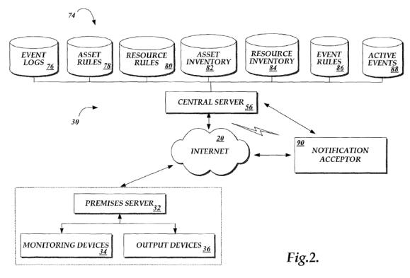
Ex. 1001, Fig. 2. Figure 2, reproduced above, "is a block diagram of an integrated information system in accordance with the present invention." *Id.* at 4:44–45. More specifically, Figure 2 shows "integrated information system 30 is a subscriber-based system allowing a number of monitoring devices within one or more premises to be processed at a single control location." *Id.* at 6:21–24.
